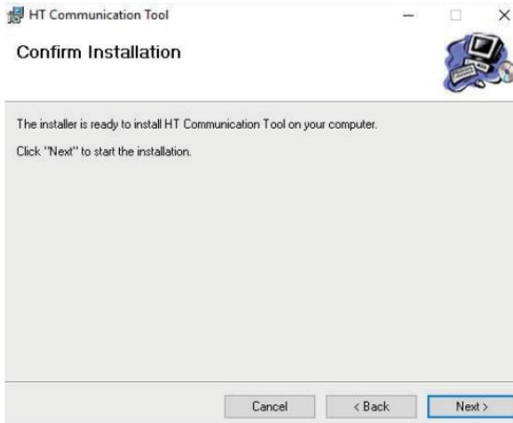
Click on “Next” to confirm installation. When the progress bar is complete, click on “Close”. A shortcut will be created on the desktop: “HT Communication Tool”.
